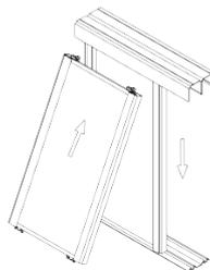
***Advice:** Before you install the doors, put a cardboard sheet on the bottom track to prevent damage to the track surface. When the doors are already in position, remove the protection cardboard.*
