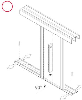
**Advice:** Before you fix the bottom track, make sure that it is positioned exactly parallel to the top track. With soft floor covering, before you fix the bottom track, cut out a strip of about 55mm in width and replace it with a 55mm timber batten. Alternatively, put a 90mm floor liner between the floor covering and bottom track. Avoid applying excessive force when tightening screws to prevent track deformation. Use flathead screws for best results.
