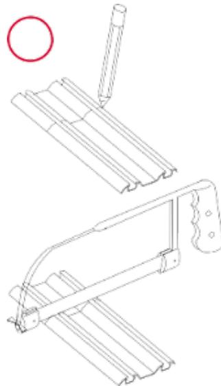
***Advice:** The tracks to be installed should be about 20mm longer than the opening width. The spare length will make it possible to avoid measurement errors and it is easier to trim. Take care not to damage the track surface whilst cutting. In order to facilitate top track cutting we advise you insert a 38mm thick wooden block.*
